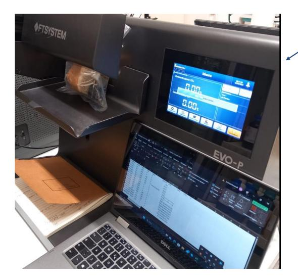
FT Systems EVO-P (spectroscopy: CO2% and O2%)
